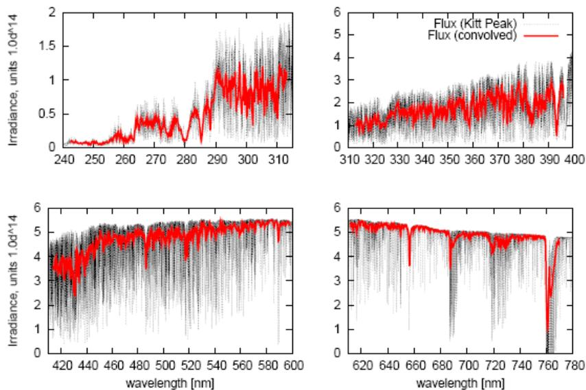
Figure 2. GOME-2 Slit function convolution of the Kitt-Peak solar spectrum.
