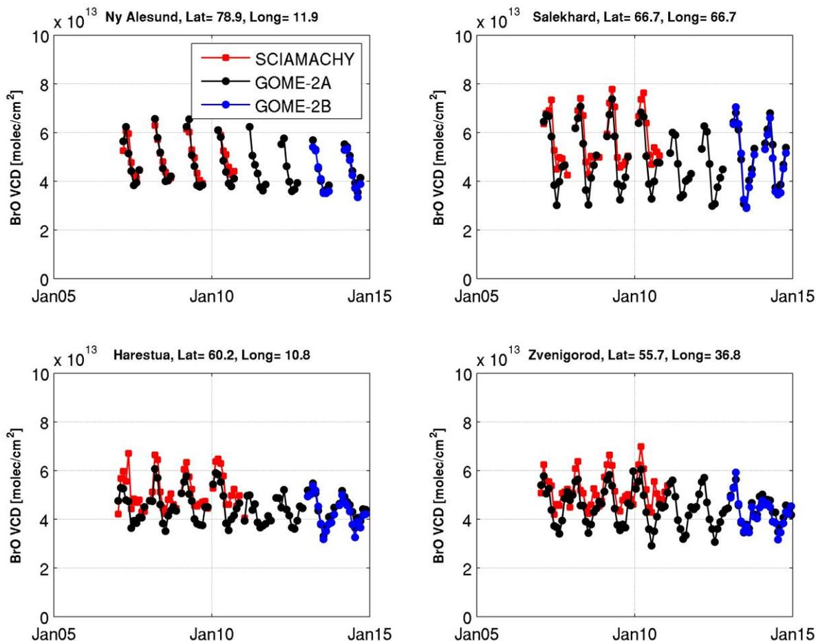
**Figure 8.** Comparison of time-series of monthly averaged BrO vertical columns retrieved from SCIAMACHY, GOME-2A and GOME-2B over the January 2007- December 2014 period, at a number of ground-based sites.
