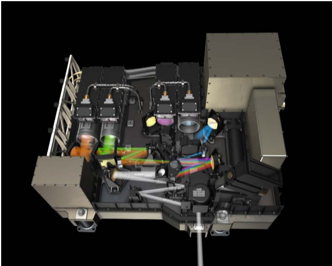
Figure 1: GOME-2 optical layout (courtesy of ESA)
