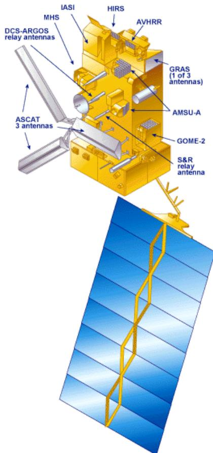
The MetOp satellite series is the core element of the EUMETSAT Polar System (EPS), developed in partnership with the European Space Agency. It carries a complement of new European instruments, as well as versions of operational instruments flown on the corresponding NOAA satellites of the USA.
