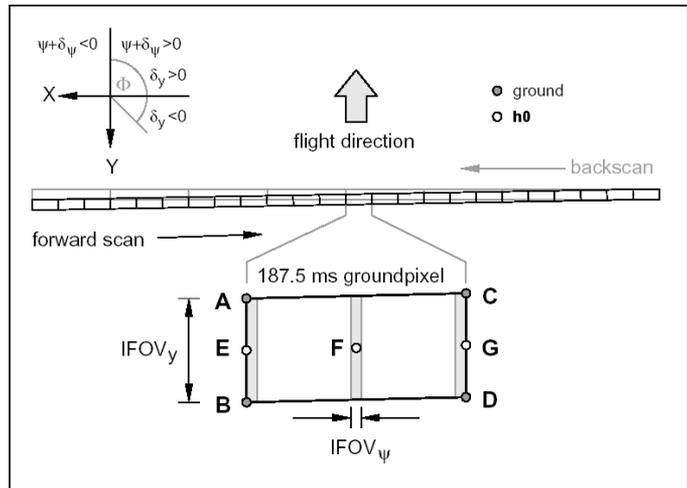
**Figure 2: Ground pixel geometry (ref: [RD3])**
