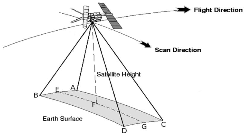
**Figure 3: Ground pixel geometry (ref: [RD3])**
