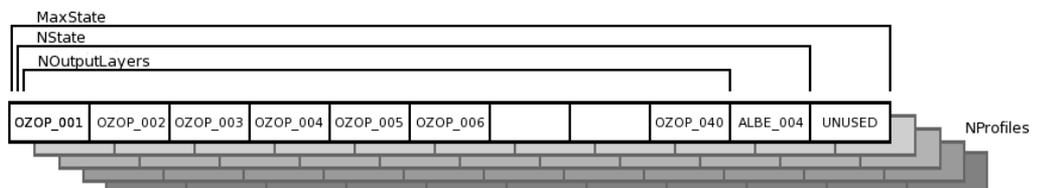
**Figure 5: The definition of the state vector within the output product**
